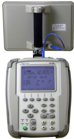
Directional Antenna Mounted on Test Set Figure 104
